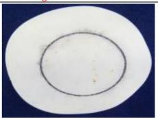
50% SK2 + 50% dem. Water STRUB from this a 6% emulsion in dem. Water STRUB created Degree of corrosion : 0 / 4
