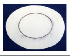
50% SK2 + 50% dem. Water STRUB from this an 8% emulsion in dem. Water STRUB created Degree of corrosion : 0 / 4
