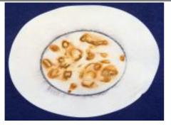
50% SK2 + 50% dem. Water STRUB from this a 5% emulsion in dem. Water STRUB created 1 Corrosion point - 1 / 4
