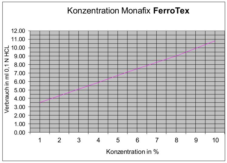
Add 0.5 ml bromophenol blue indicator solution to 50 ml liquid and titrate with 0.1N HCL until the color changes (to gray-green). The consumption of ml HCL is plotted on the Y-axis and the concentration of MONAFIX Ferrotex is read on the X-axis.
